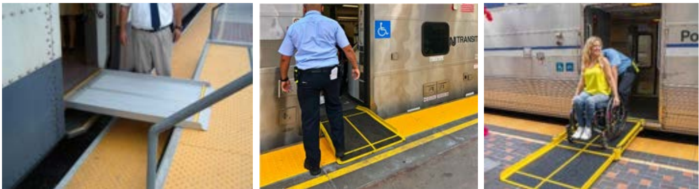
Figure 23. Deployed Bridge Plates and Bridge Plate Ramps (Photos courtesy of SBCTA, Wikipedia and NJ Transit, and LOSSAN Agency)
