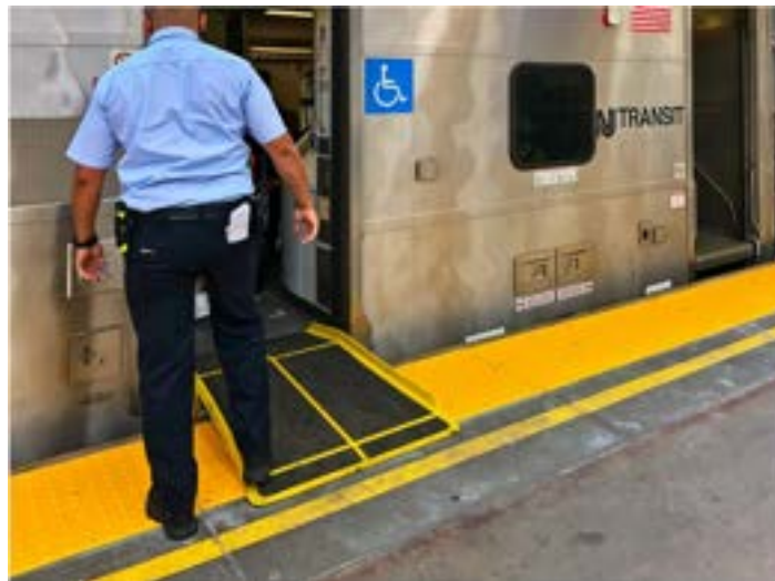
Figure 20. Deployed Bridge Plate (Photo courtesy of Wikipedia and NJ Transit)
