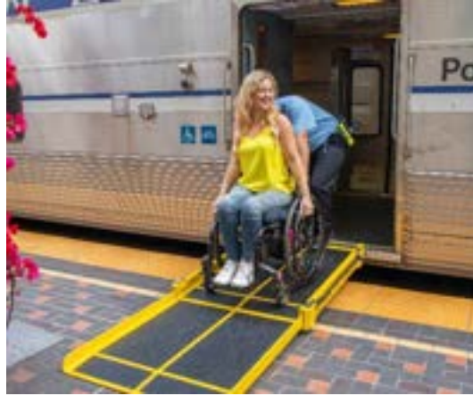
Figure 21. Deployed ADA Ramp (Photo courtesy of LOSSAN Agency)
