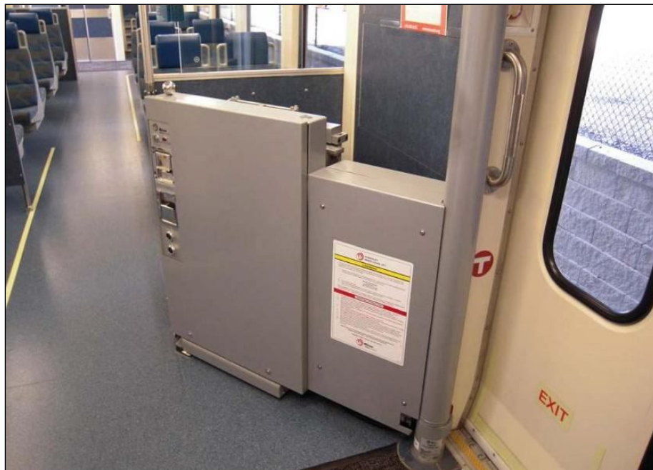
Figure 25. Car-borne Conductor Deployed Automated Ramps Source: Metro Transit, 2010
