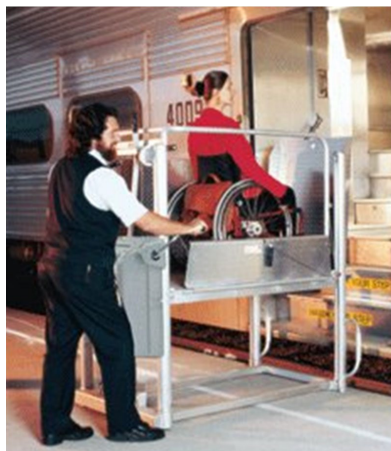
Figure 22. Portable Wheelchair Lift for Horizon and Comet Car Access (Photo courtesy of Adaptive Engineering Inc.)
