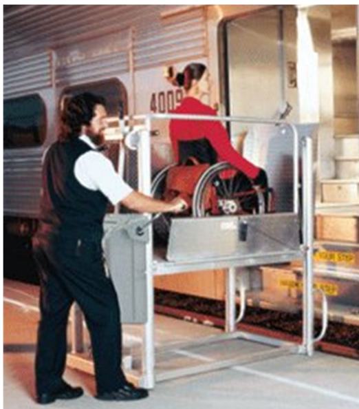
Figure 28. Portable Wheelchair Lift for Horizon and Comet Car Access
