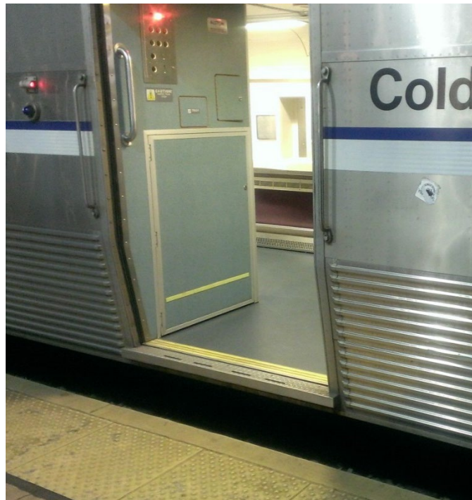
Figure 15. Recessed Doors on Amtrak Surfliner Cars
